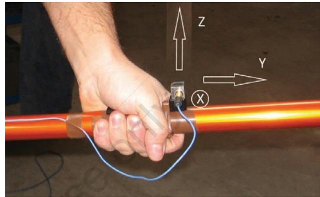
**Figure 3. Vibration measurement directions on the harvester pole.**
