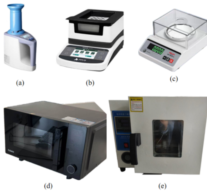
Figure 2. Experimental equipment. a) Grain moisture meter. b) Halogen moisture meter. c) Delixi Electric LCD electronic analytical balance. d) Galanz G90F25YeSXLV-ADG0 microwave drying experimental station. e) Mingyue MY-382 electric thermostatic drying oven used for laboratory hot-air drying.
