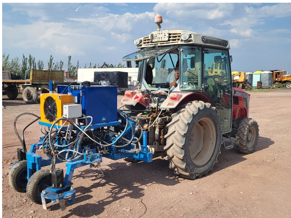
Figure 7. An industrial prototype of a universal rotary tiller developed by a scientific team (ANAU).
