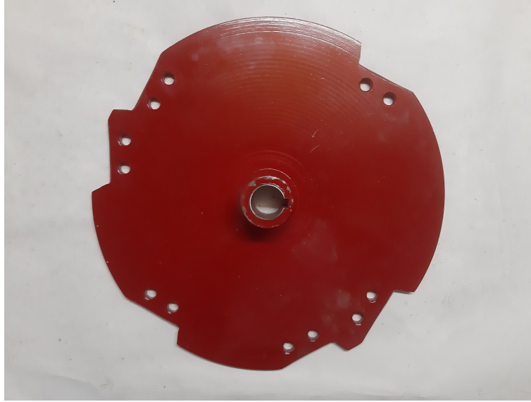
Figure 2. General view of the rotary tiller experimental disc used in the experiments (example D = 400 mm).
