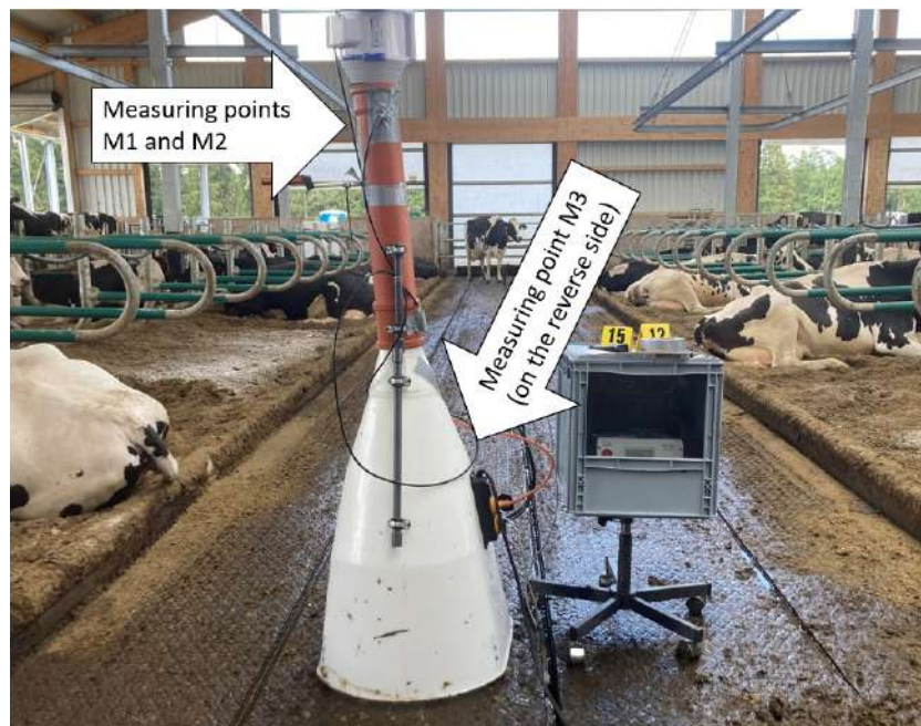
Figure 2. Dynamic flux chamber with multi-gas monitor in a plastic box.
