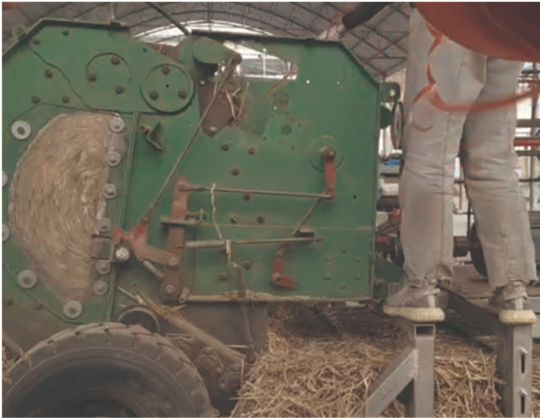
Figure S6. Experimental verification of the cone frustum-steel roll baling mechanism. a) Manual assistance for rope winding. b) Complete straw bales.
