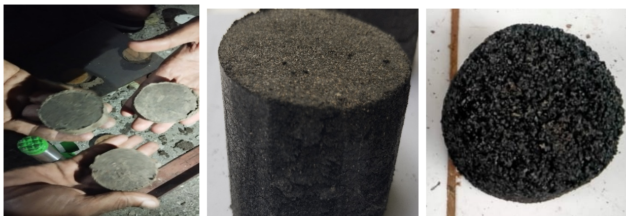
Figure 2. Candle nut shell briquettes produced at different particle sizes: 20 mesh (left); 40 mesh (middle); 60 mesh (right).
