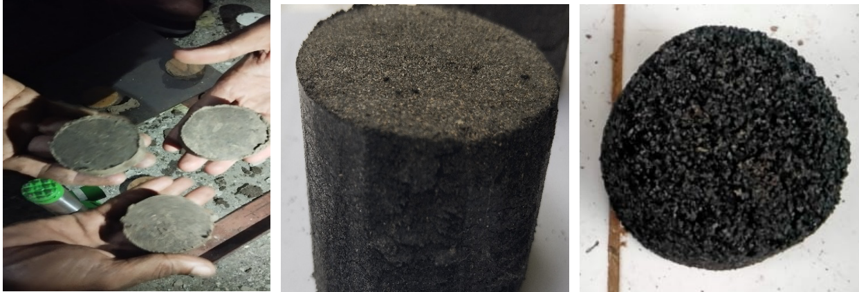
Figure 2. Hazelnut shell briquettes produced at different particle sizes: 20 mesh (left); 40 mesh (middle); 60 mesh (right).
