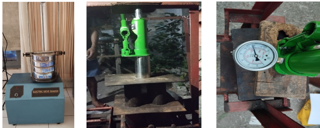
Figure 1. Equipment employed in briquette production: sieve shaker (left); hydraulic press (middle); briquette mold system (right).
