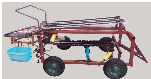
Figure 10. Side view of the developed poppy harvesting prototype showing the carrier and pulling brush systems, circular cutting blades, and capsule collection unit.
