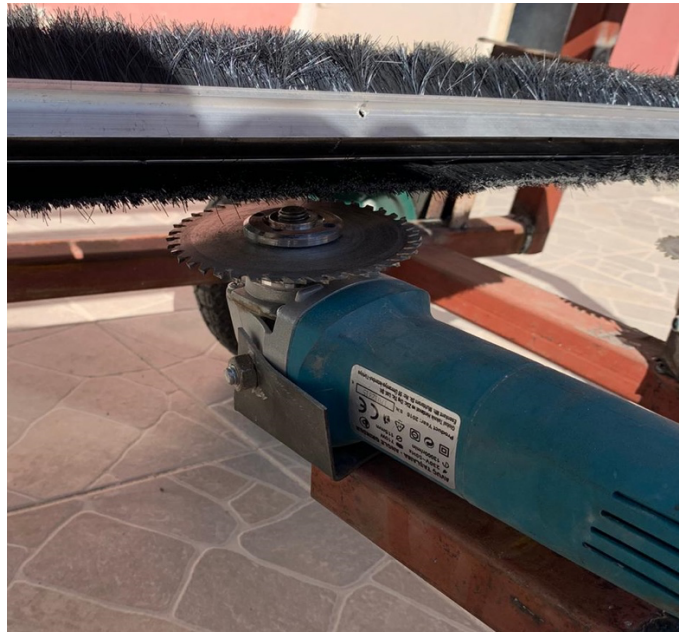
Figure 5. Cutting blade placement.
