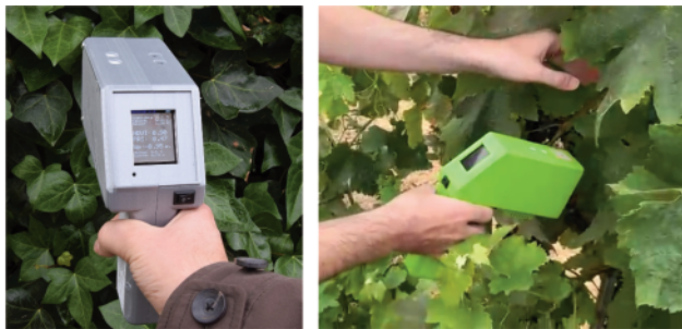
Figure 3. Handheld prototypes for rapid assessment of tree stress.
