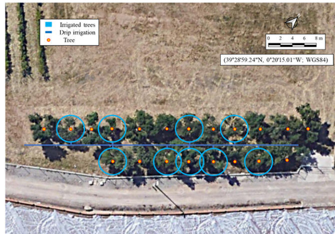
Figure 2. Experimentation site and irrigation design.
