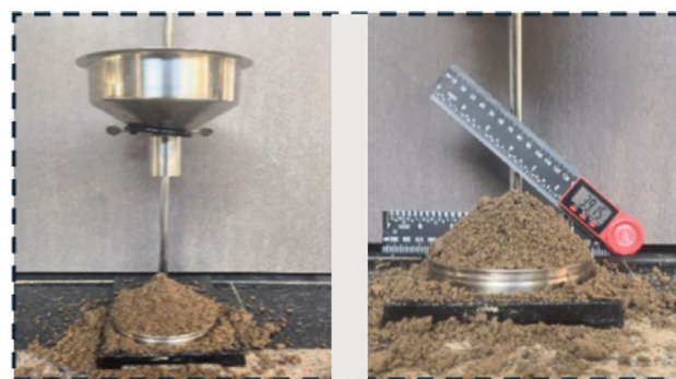
Figure 5. Soil angle of repose test.
