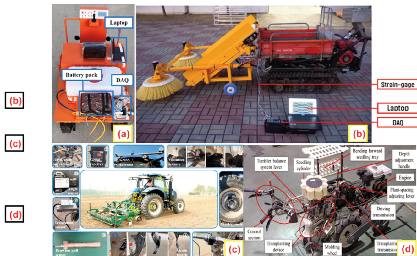
Figure 2. Example of load measurement systems applied in agricultural machinery. a) Retrieved from: Hwang et al. Agriculture 2024;14:416; with permission. b) Retrieved from: Kim et al. Agriculture 2022;12:1071; with permission. c) Retrieved from: Zhang et al. , Agriculture 2024;14:1604; with permission. d) Retrieved from: Markunningsih et al. Agriculture 2023;3:588; with permission.
