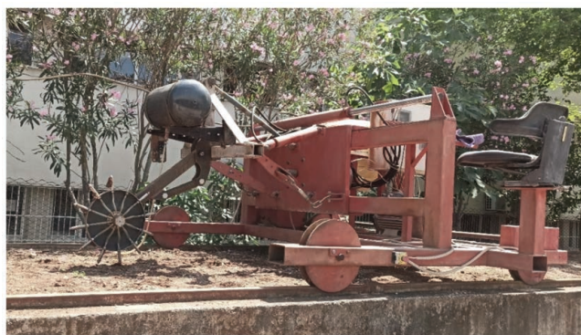
Figure 4. Installed Point Injection Liquid Manure System with small tank and air compressor on soil bin channel's moving carriage.
