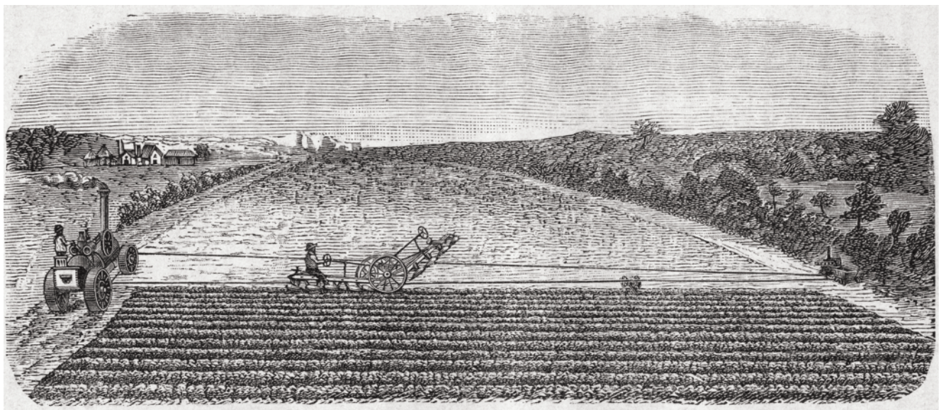
Figure 2. Fowler plowing system, complete with locomotive and anchor wagon (MAIC, 1885, p. 24).
