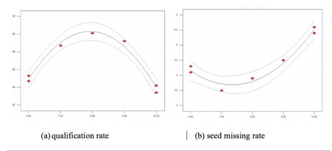
Figure 10. Effect of the angle of the seed cleaning plate on the qualification rate and the seed missing rate.
