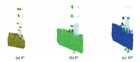
Figure 9. Clear seeding simulation results in different angles of seed cleaning plate.
