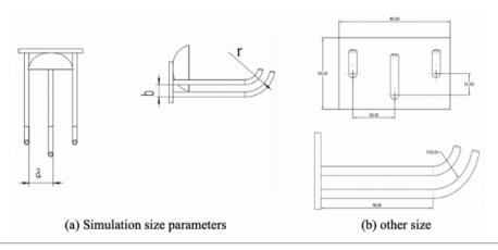
Figure 3. Structural parameters of seed picking claw.
