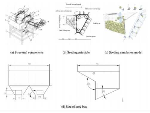
**Figure 2.** Main structure of seed metering device. 1. frame; 2. seed box; 3. support plate; 4. driving shaft; 5. seed picking claw; 6. seed preventing plate; 7. driven shaft; 8. seed clearing plate; 9. motors; 10. reducer; 11. bearing support; 12. driven shaft.
