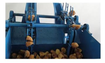
Figure 12. Comparative experiment of potato seed metering device.
