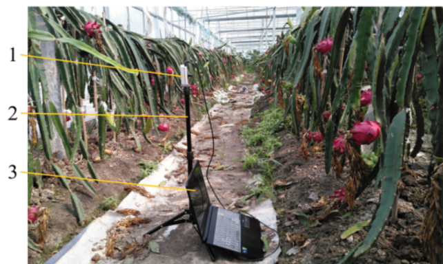
Figure 1. Pitaya trees in the densely planted commercial orchard and image acquisition device. 1, D435i depth camera; 2, tripod; 3, notebook computer.
