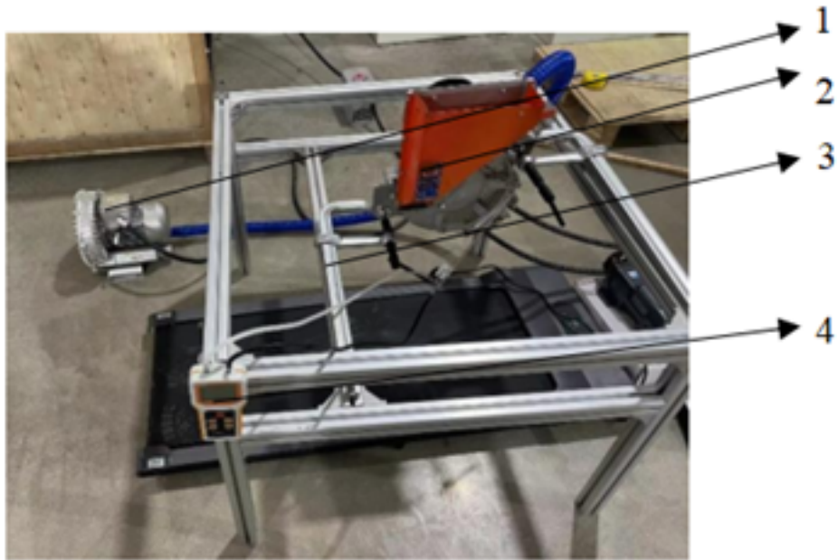
Figure 5. Test bench for the air-suction precision wheat seed metering device. 1. Wind turbine control system; 2. pneumatic wheat precision seeder; 3. seeder performance testing stand; 4. wind speed and airflow meter.
