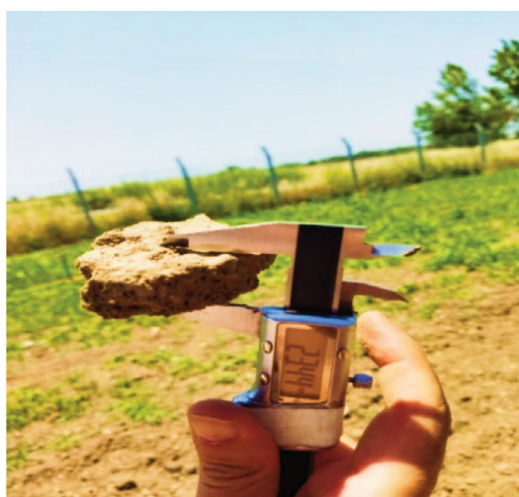
Figure 2. The measurements of soil crust thickness.
