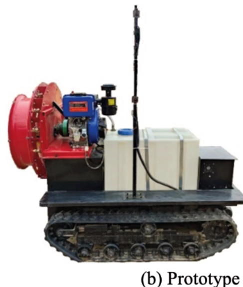
Figure 1. Self-propelled target spraying machine. 1. Control box; 2. Operation monitoring module; 3. Brushless DC motors; 4. Tracked chassis; 5. Range extender; 6. Battery pack; 7. Sprayer tank; 8. Solenoid control valve; 9. Centrifugal fan; 10. Infrared laser sensors; 11. Diesel engine; 12. Plunger pump; 13. High pressure nozzles.
