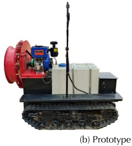
Figure 1. Self-propelled target spraying machine. 1. Control box, 2. Operation monitoring module, 3. Brushless DC motors, 4. Tracked chassis, 5. Range extender, 6. Battery pack, 7. Sprayer tank, 8. Solenoid control valve, 9. Centrifugal fan 10. Infrared laser sensors, 11. Diesel engine, 12. Plunger pump, 13. High pressure nozzles
