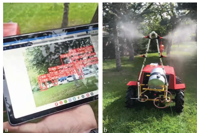
Figure 4. Artificial intelligence-based tree recognition. a) Artificial intelligence application. b) Operation of the robotic spraying mechanism.
