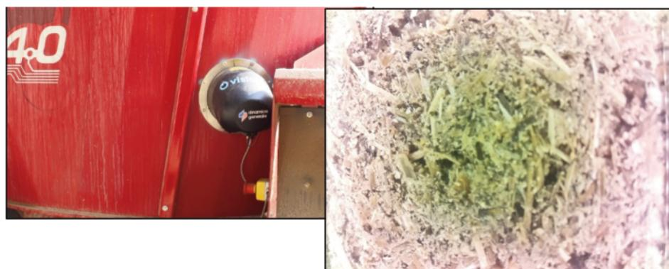
**Figure 1.** Details of the sensor installation for fibre length and TMR homogeneity assessment (on the left) and a screenshot of the captured image (on the right).
