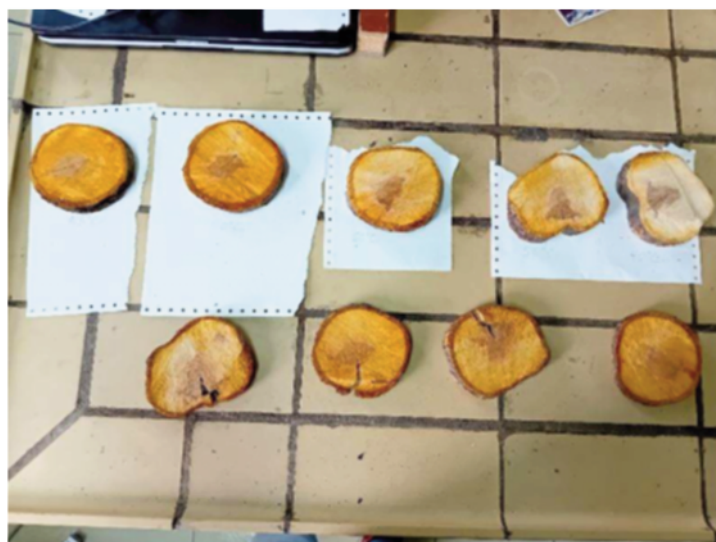
Figure 1. Wood discs samples for experimental drying process.
