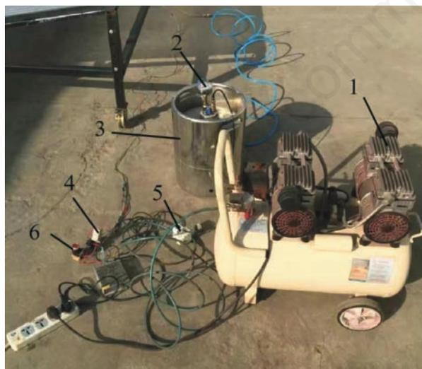
**Figure 5.** Photographs of the test site. 1. Air compressor; 2. pressure gauge; 3. water tank; 4. timing relay; 5. regulator; 6. switch.
