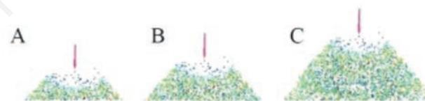
**Figure 9.** Spray pattern under different spraying conditions. **A)** Spraying height: 0.5 m - tilt angle: 1°. **B)** Spraying height: 0.6 m - tilt angle: 1°. **C)** Spraying height: 0.8m - tilt angle: 1°..
