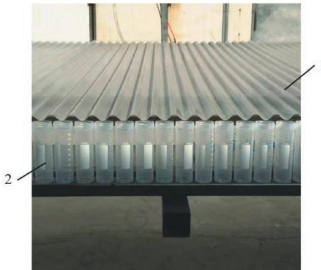
**Figure 8.** Droplet collection device. 1. Wave through; 2. test tube diagrams.
