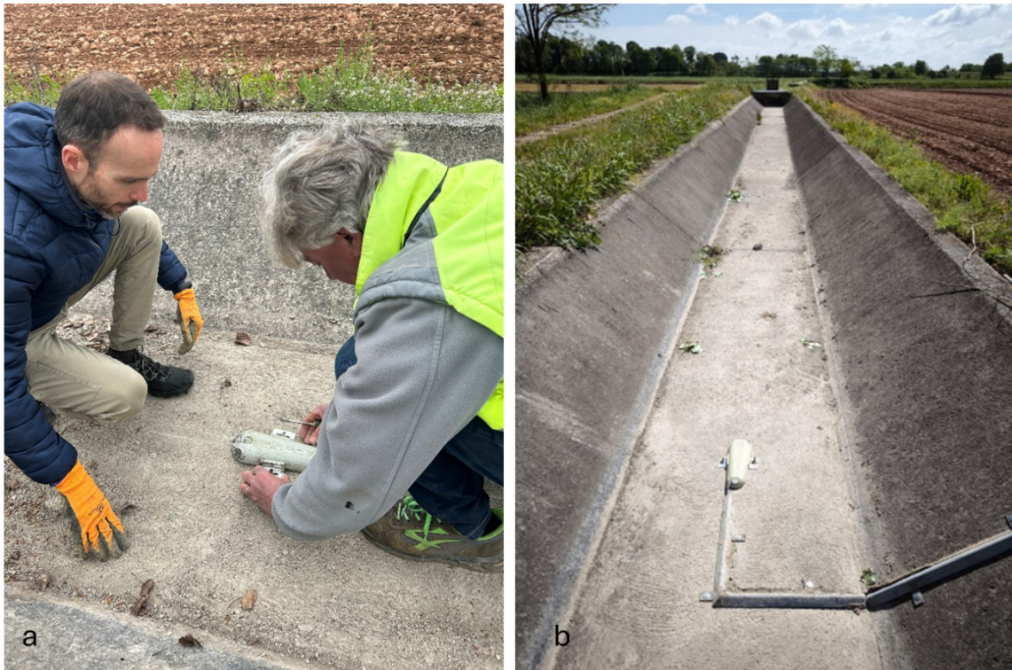
Figure B. Area-velocity meter (Sontek-IQ series, standard model, Xylem) installation moment (a) and device location inside the distribution canal at and of installation (b).
