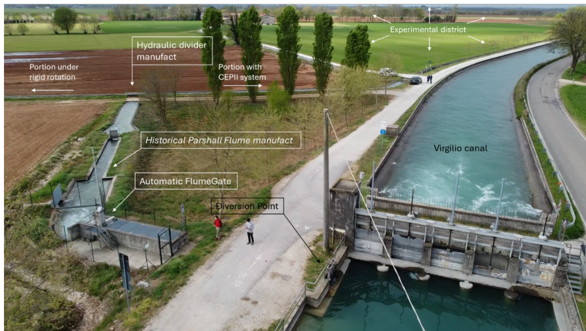
Figure 1. Aerial photograph of the head of the Ponte Trento irrigation district. The picture shows the Virgilio canal, the diversion point, the hydraulic divider, and the experimental part of the district where CEPII system was adopted.
