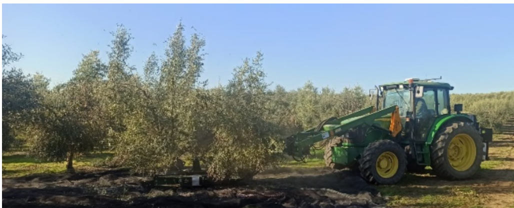
Figure 1. Orchard and trunk shaker used in the experiment.
