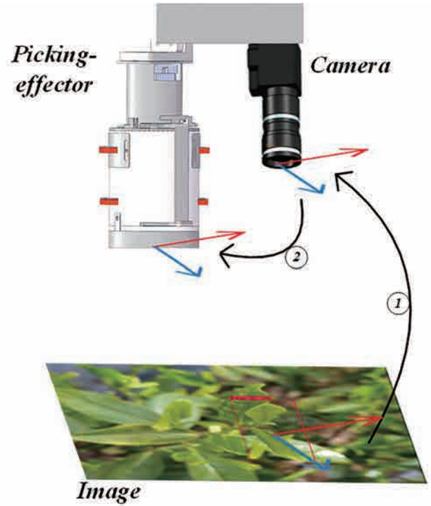
Figure 5. Coordinate system transformation. 1, the pixel coordinate system to the camera coordinate system; 2, the camera coordinate system to the picking effector coordinate system
