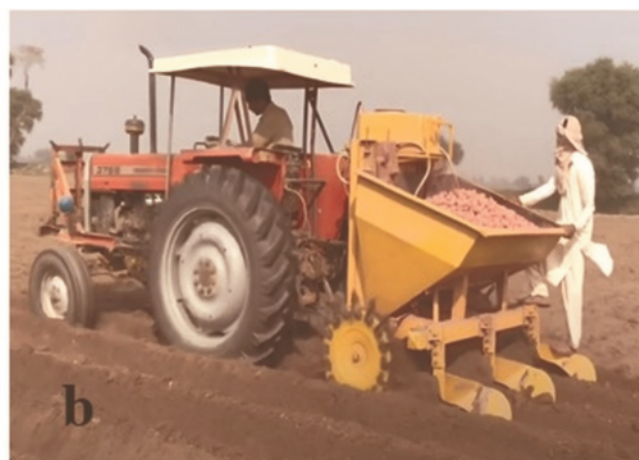
Figure 6. Sowing and planting implements/ machines a) Ride on rice nursery rice transplanter manufactured by Kubota; b) Locally manufactured tractor mounted potato planter.
