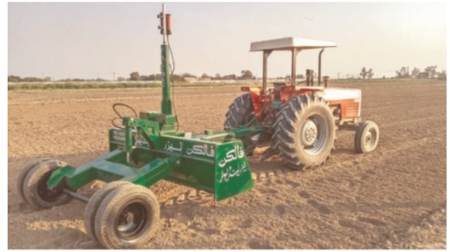
Figure 9. Locally manufactured Laser Land Leveller in a farmer's field. These LLL are equipped with imported transmitters mostly imported from USA and China.
