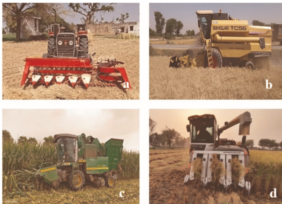
Figure 8. Harvesting machinery. a) Locally manufactured tractor mounted wheat reaper; b) New Holland conventional wheat combine harvester; c) Chinese self-propelled maize cob picker manufactured by Dafeng; d) Kubota built half feed paddy harvester working in paddy fields.
