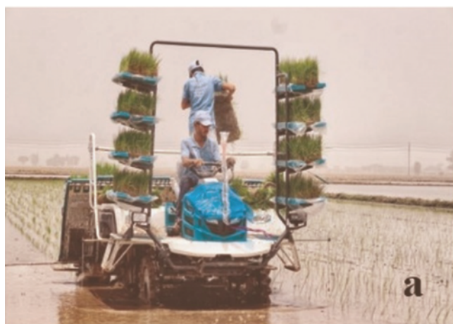
Figure 6. Sowing and planting implements/ machines a) Ride on rice nursery rice transplanter manufactured by Kubota; b) Locally manufactured tractor mounted potato planter.
