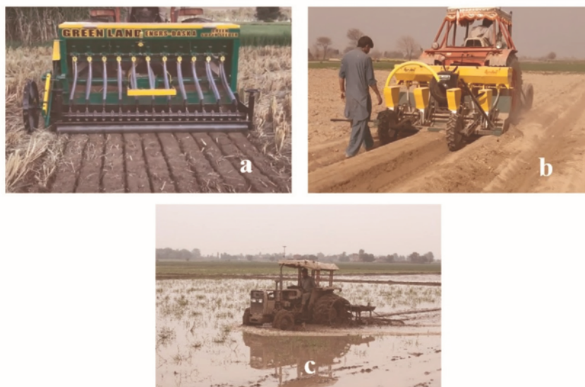
Figure 5. Land preparation implements/ machines. a) Pneumatic planter for maize sowing manufactured locally; b) Pak seeder for land preparation and sowing of wheat developed by AMRI and local manufacturing firm Greenland Engineers; c) Land preparation operation (puddling) for rice nursery transplantation using locally manufactured tine cultivator.
