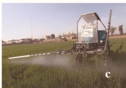
Figure 7. Interculture implements/ machines. a) Locally manufactured tractor mounted row interculture implement; b) Locally manufactured tractor mounted boom sprayer; c) Advanced self-propelled boom sprayer manufactured by Kubota.
