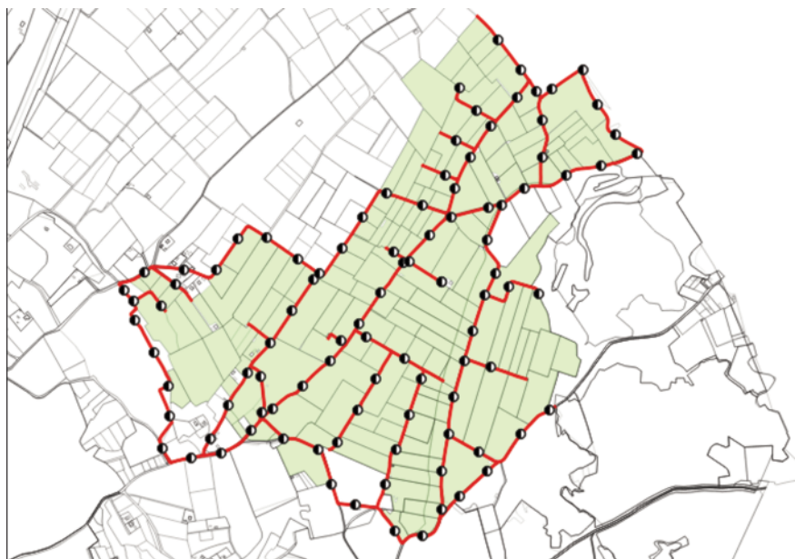
Figure 3. Equidistant candidate hydrants on irrigable surface.
