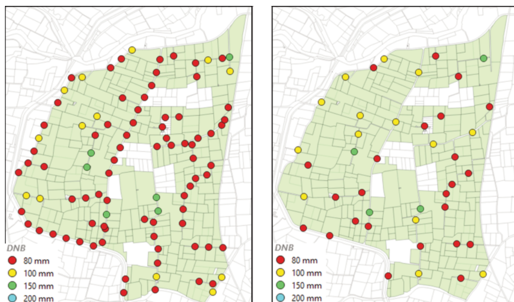
Figure 6. Difference in the number of hydrants between initial (left) and final (right) solutions for each type of DN.
