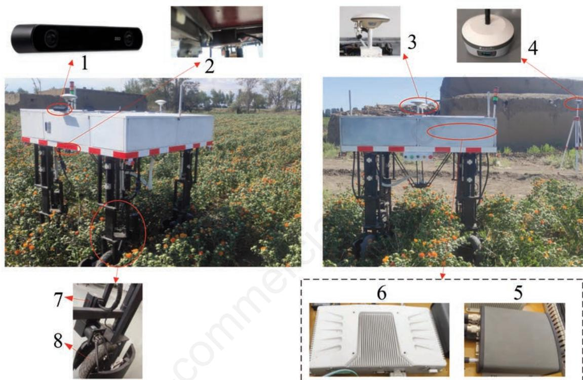
**Figure 1.** Safflower picking robot structure: 1) binocular camera; 2) inertial measurement unit; 3) satellite antenna; 4) satellite base station; 5) satellite receiver; 6) industrial computer; 7) servo motor; 8) drive wheel.
