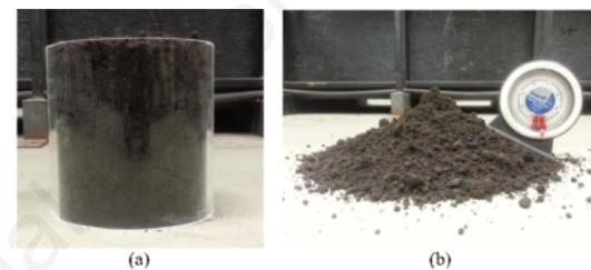
**Figure 3.** (a) A cylinder filled with soil particles is used to measure the angle of repose, (b) accumulations of soil particles on a wall (Qi *et al.*, 2019).
