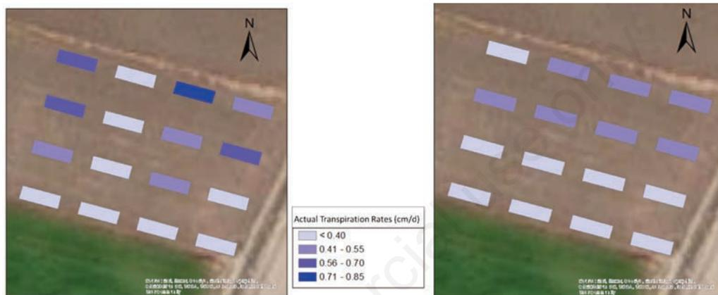
**Figure 7.** Colour-graduated maps of the canopy transpiration rates,  $T_{a,c}$ , obtained as upscaled leaf-scale transpiration on the left and of the macroscopic transpiration rates obtained from FLOWS model,  $T_{a,m}$ , on the right. The canopy transpiration rates in the maps represent the averages of two daily transpiration rate measurements carried out on 5 and 10 August 2020.
