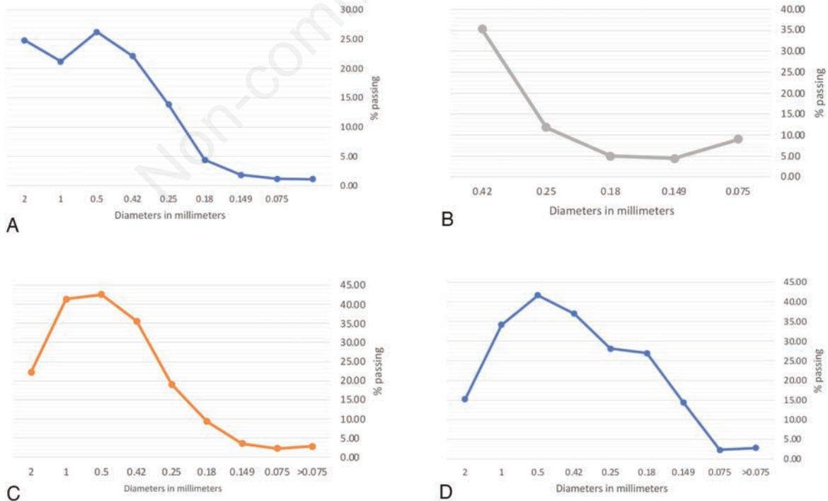
**Figure 1.** Particle size distribution of Florida soil (FS) (A), clay (B), the size distribution of FSM (C), the particle size of the final mix (including sand) (D).
