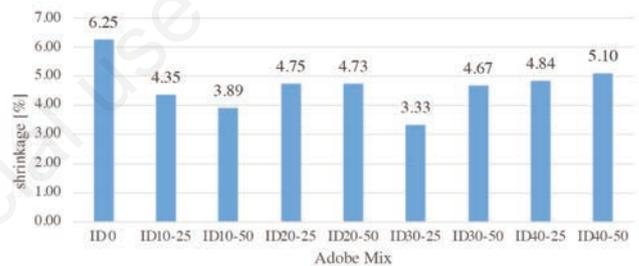
Figure 9. Shrinkage rate for prismatic samples.
