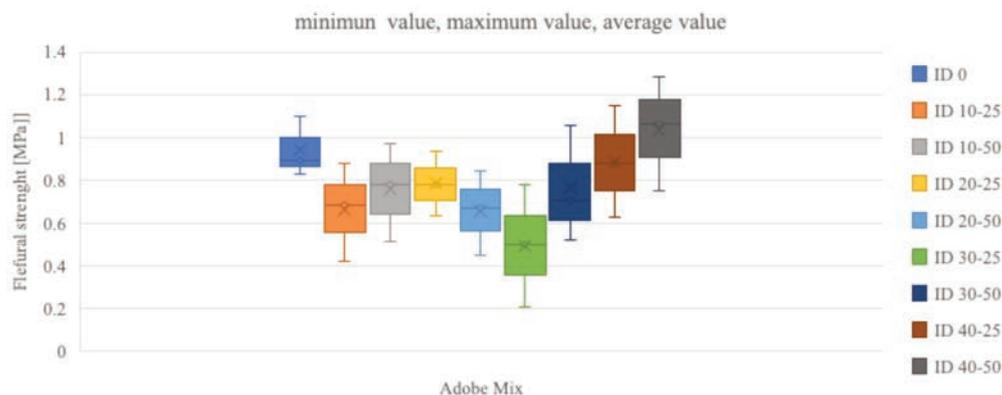
Figure 6. Average values of flexural strength of the adobe mix, including minimum and maximum values for each mix.
