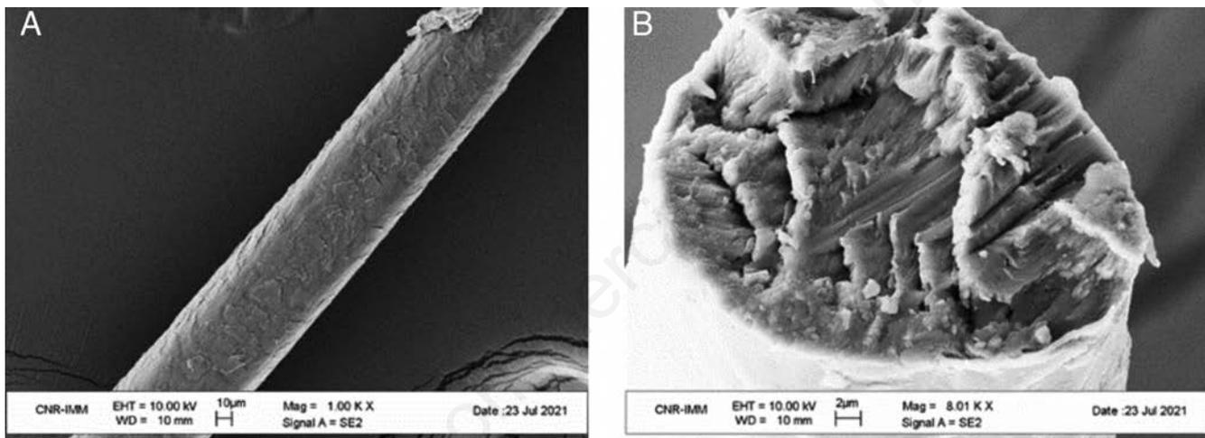
**Figure 2.** Scanning electron microscope analysis of sheep wool fibre surface (A) and transversal section (B).
