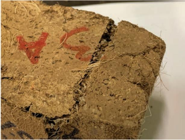
**Figure 12.** Composite specimens after compression test.
