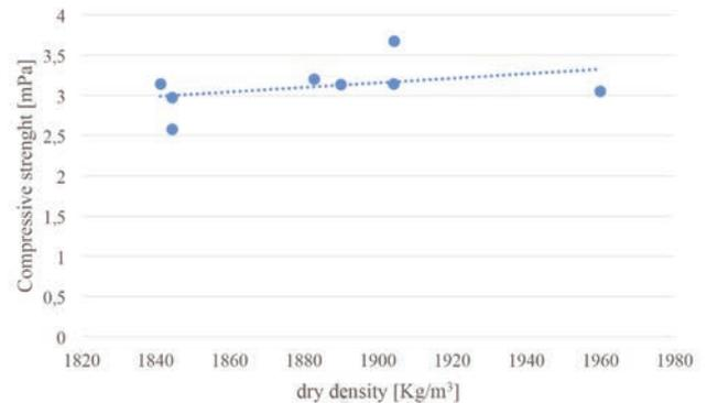
Figure 8. Correlation between dry density and compressive strength.
