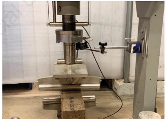
Figure 4. A sample ready for the flexural test.
