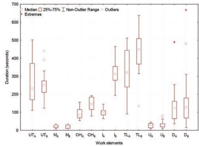
Figure 3. Summary statistics of work elemental time of TAF 690 PE cable skidder.
