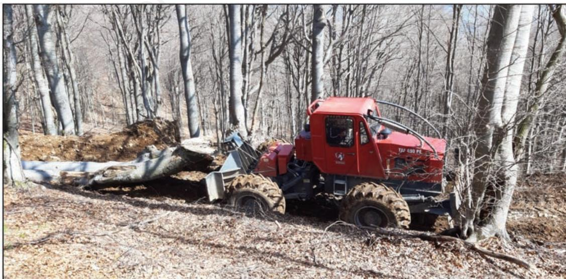
**Figure 2.** The articulated 4WD TAF 690 PD cable skidder used in the test.
