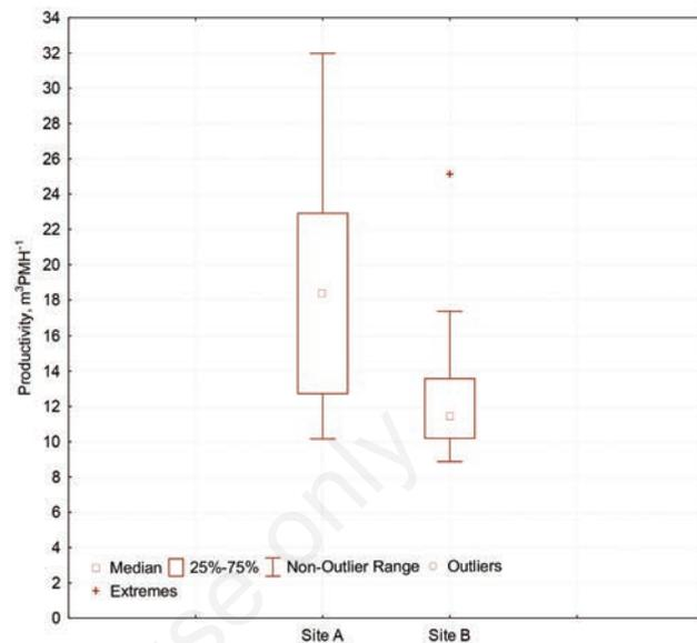
**Figure 4.** Summary statistics of the skidding productivity for the two sites. PMH, productive machine hour.
