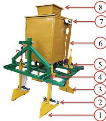
Figure 3. The cardboard injection prototype: 1- furrow openers; 2- cardboard distributor; 3- coverage unit; 4- chassis; 5- lateral slider; 6- cardboard mixing unit; 7- operating switches; 8- hopper.
