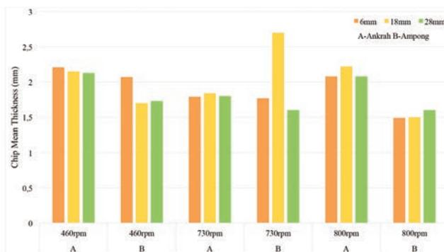
Figure 8. Mean thickness (mm), operating speed (rpm), and chipping clearance (mm) of *Ankrah* 48AH and *Ampong* 48AH.
