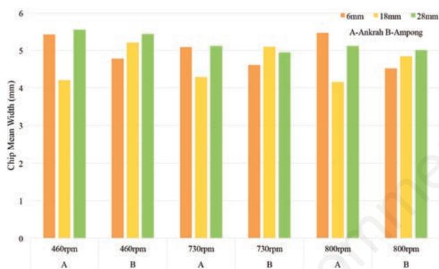
Figure 5. Mean width (mm), operating speed (rpm), and chipping clearance (mm) of *Ankrah* FH and *Ampong* FH.
