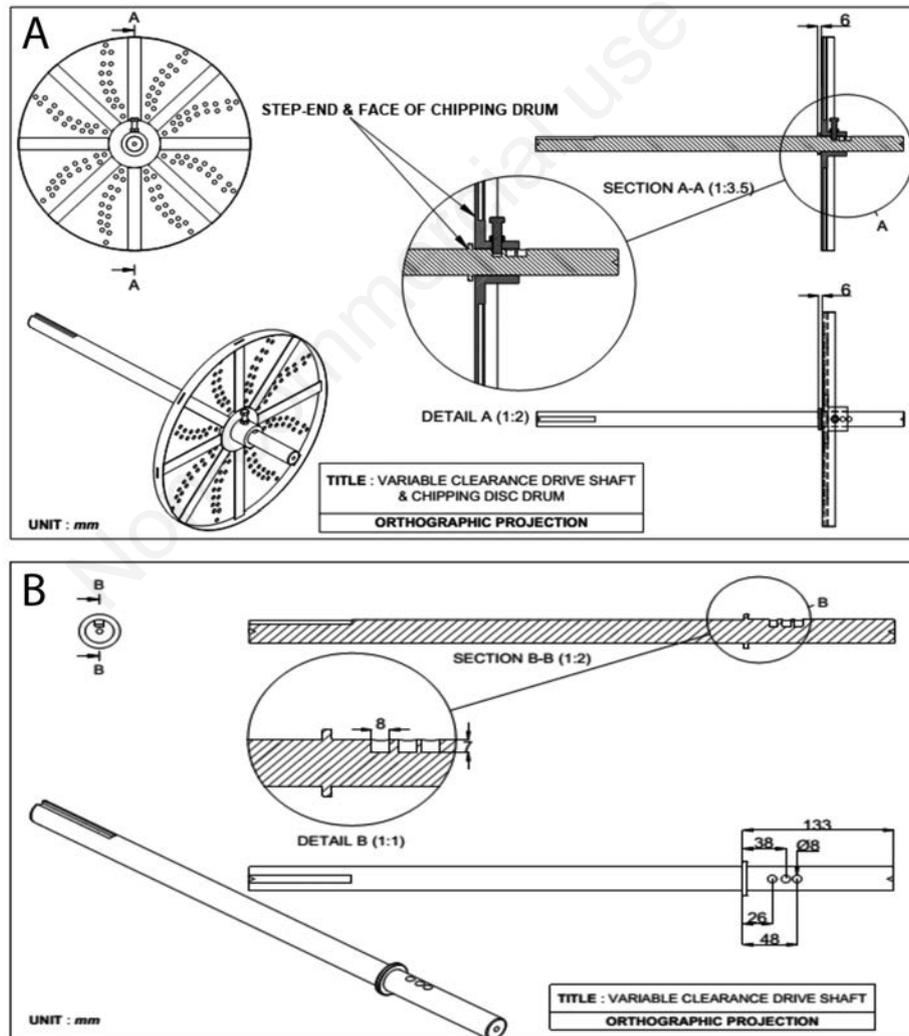
Figure 2. A) Orthographic projection views of the variable clearance drive shaft and chipping disc drum; B) orthographic projection views of the variable clearance drive shaft.
