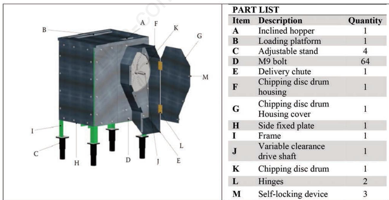
Figure 1. Isometric view of the variable clearance.
