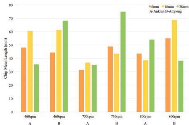
**Figure 3. Chip mean length (mm), operating speed (rpm), and chipping clearance (mm) of *Ankrab* FH and *Ampong* FH.**
