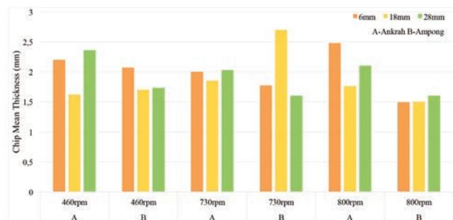
Figure 7. Mean thickness (mm), operating speed (rpm), and chipping clearance (mm) of *Ankrah* FH and *Ampong* FH.
