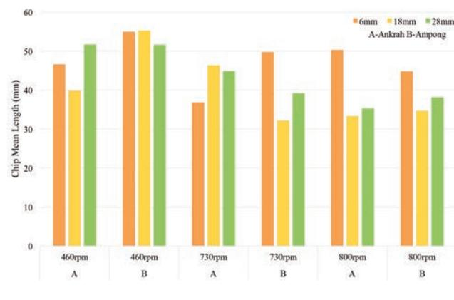
**Figure 4. Chip mean length (mm), operating speed (rpm), and chipping clearance (mm) of *Ankrab* 48AH and *Ampong* 48AH.**
