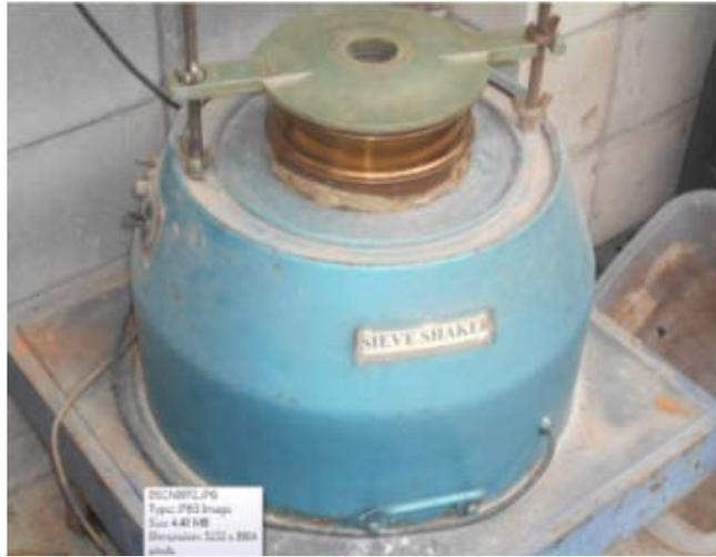
**Appendix Figure 8. Mechanical sieve shaker used for sieving the samples.**
