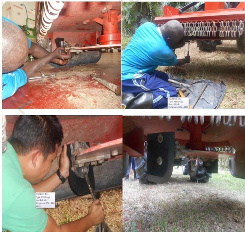
**Appendix Figure 3. Replacement of tractor mounted mulcher blades.**
