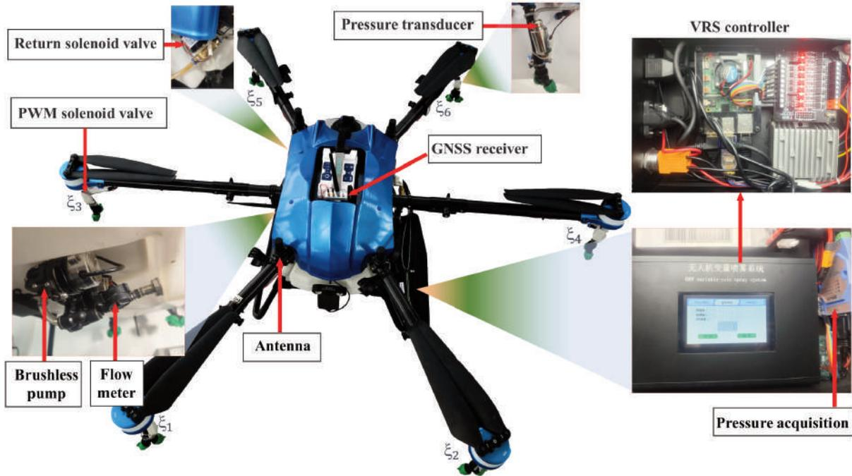
Figure 1. A six-rotor electric unmanned aerial vehicle with variable-rate spray system.
