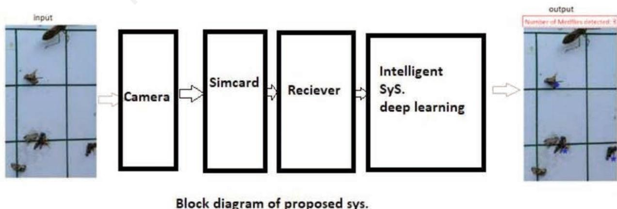
Figure 4. Intelligent system architecture for Medfly detection.
